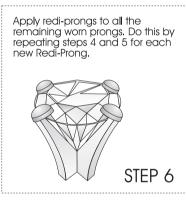
If needed flow a small drop of gold solder to back edge of prong to blend old prong to new Redi-Prong. Repeat this step on each prong.
